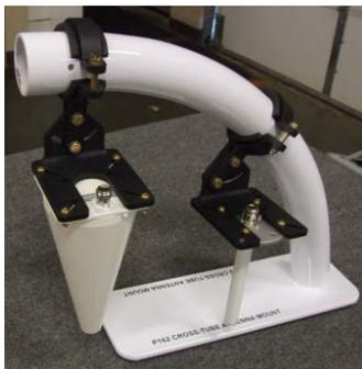
Example of antennas mounted on a cross-tube mount.
